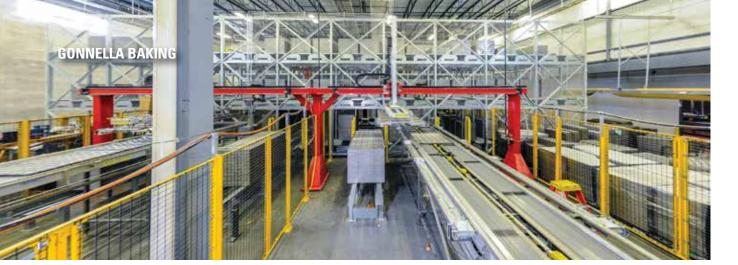
The robotic pan handling system streamlines changeovers from seven to three minutes. Its mechanical fingers delicately pick up multiple pans at a time, then the two robots stack or unstack them while production shifts from one product variety to another.
