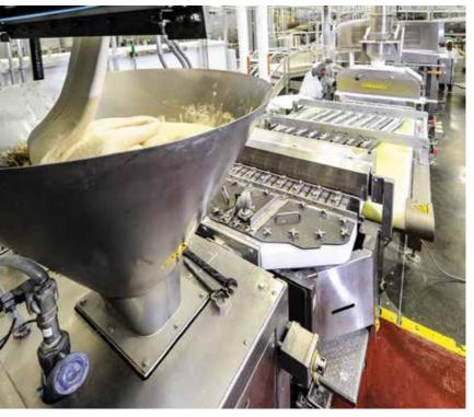
The high-speed divider and makeup system turns out dough balls with pinpoint accuracy that has helped increase the bakery's yield.
